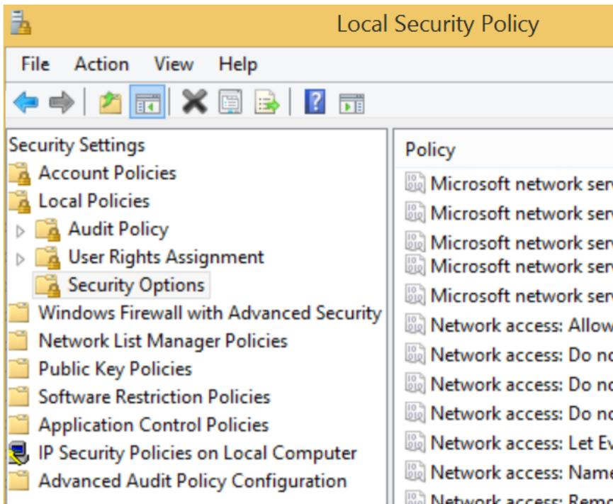
Step 4. Check the Security setting of Network Access: Sharing and security model for local accounts is “Classic”
