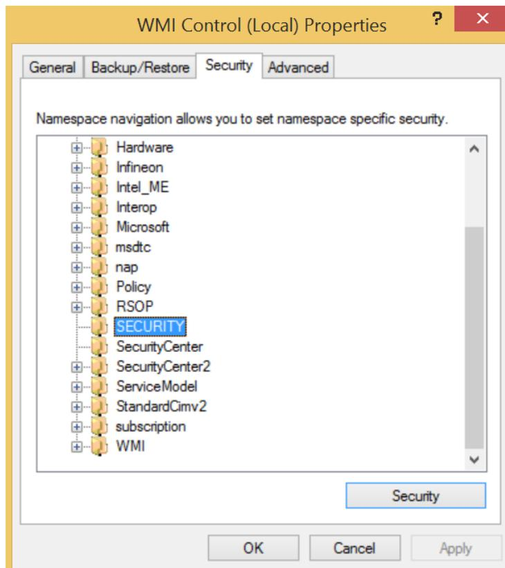
Step 5. Ensure the [Execute Methods](#), [Provider Write](#) and [Enable Account](#) enabled in [Permission for Authenticated Users](#).
